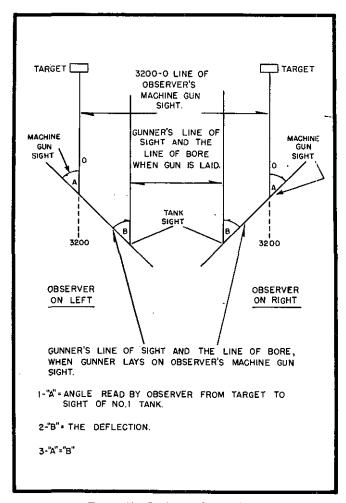
FIGURE 41.-Laying tanks parallel.
