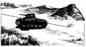
FIGURE 22.—Desired trajectory—laying on center of target.
