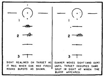
FIGURE 24.—Automatic correction method.
