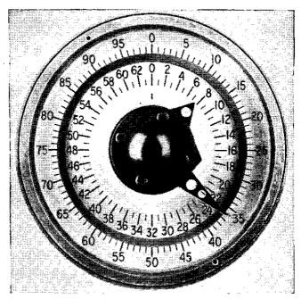
FIGURE 38.—Azimuth indicator.
