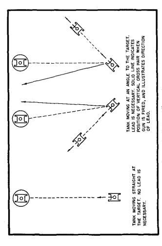
Figure 29,-Firing while moving.
