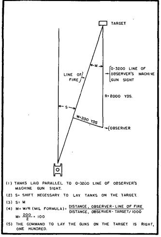
FIGURE 42.—Correcting for position of observer.
