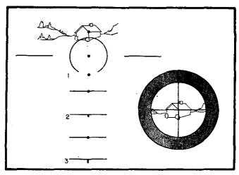
Figure 11.—When adjusting sights, use horizontal and vertical edges to insure that the gun and sight are laid on precisely the same point.
