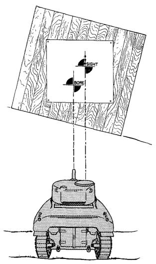
FIGURE 12.—Rotate the testing target in a vertical plane (see par. 42.)
