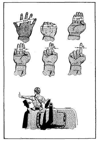
FIGURE 44.—Measuring angles with the hand.
