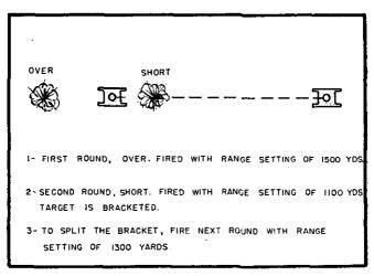
FIGURE 25.—Bracketing the target.
